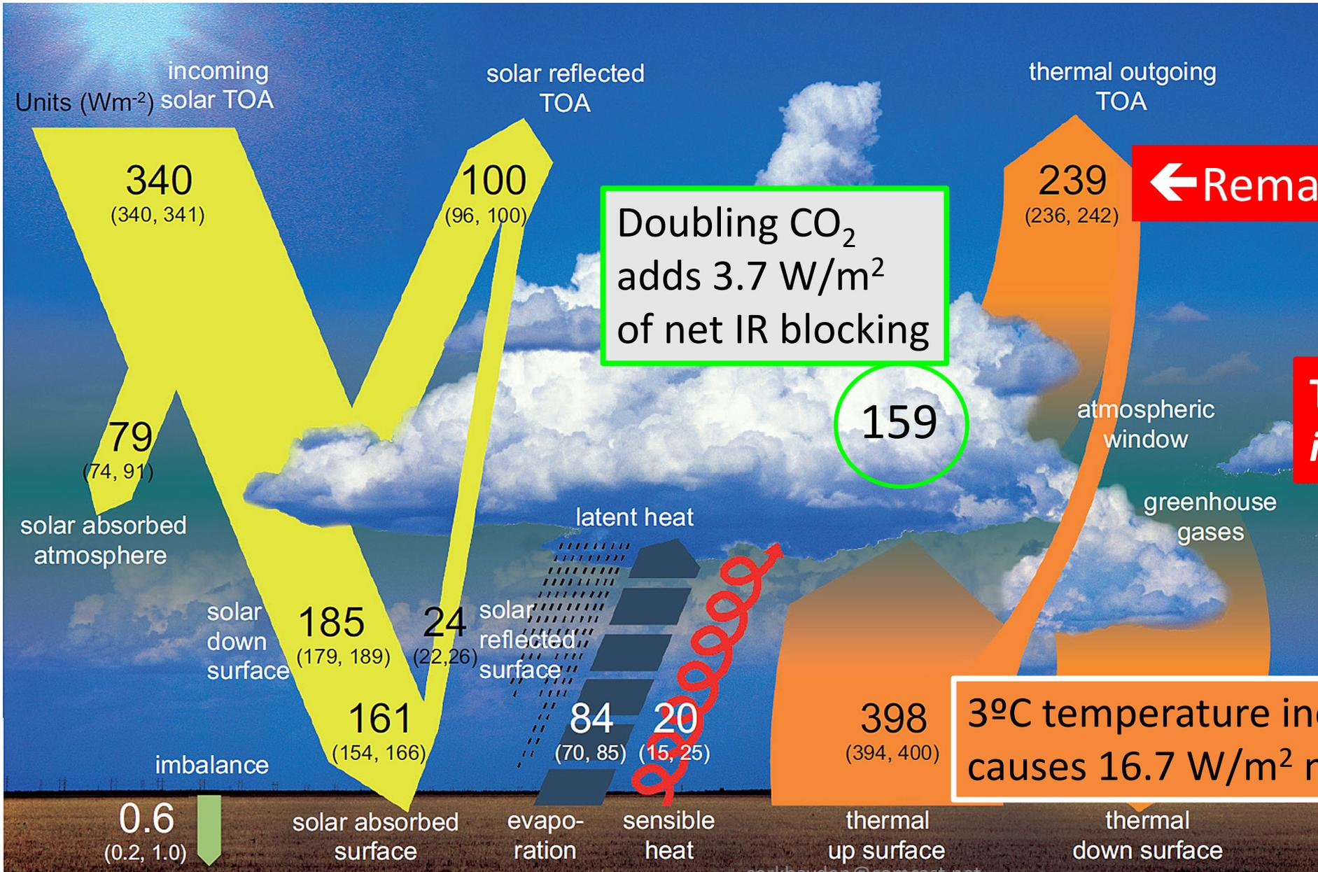
Doubling CO<sub>2</sub> adds 3.7 W/m<sup>2</sup> of net IR blocking
